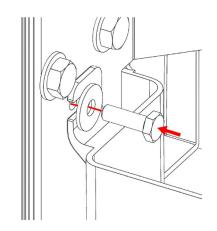
**11.** Seal all possible joints on the parts, aluminium profiles and column reinforcement brackets.
