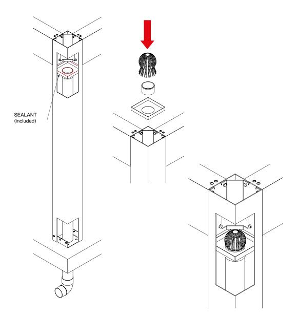
Finally, apply the sealant (included) all around the perimeter of the collecting tray and the adapter, as shown in the picture (sealant in red), and insert the universal leaf guard into the adapter.
