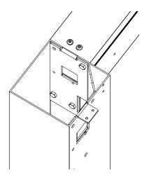
Screw two ULS ISO 7380 M6x16 screws into the column fitting at the top of the beam before fitting the other screws
