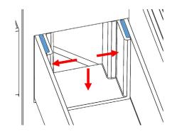
**5.** The corner between the extension piece and the gutter must then be sealed.
