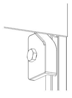
On the left side of the column, clip the profile onto the clipping rubber from the bottom to the top.
