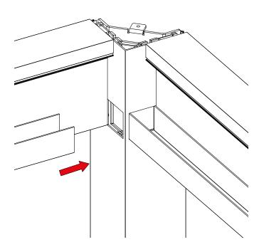
Check that all the "U" profile holes match the M6 machined ones on the beam. If all of them match, apply the sealant between the "U" profile and the beam after screwing the profiles with the USL (ISO 7380) A2x16 screws.
