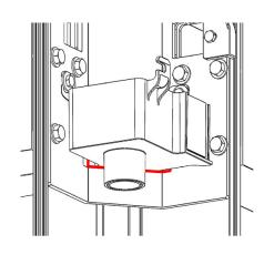
**10.** Seal all the joints between the gutter extensions and the collecting tray (marked in red in the picture) with silicone.
