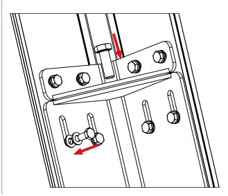
**3.** Screw a coupling piece of the cover profile onto the base L using a DIN 933 A2 M6x10 screw. (3)
