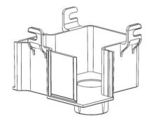
**9.** Place the collecting tray under the gutter extensions.
