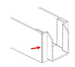
**2.** Install the piece into the gutter from the inside of the column, taking care not to remove the silicone in the process.
