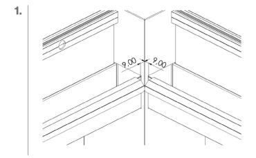
Fit the perimeter LED corner piece shown in the picture on the right to the **corners of the pergola with a mitre**.
