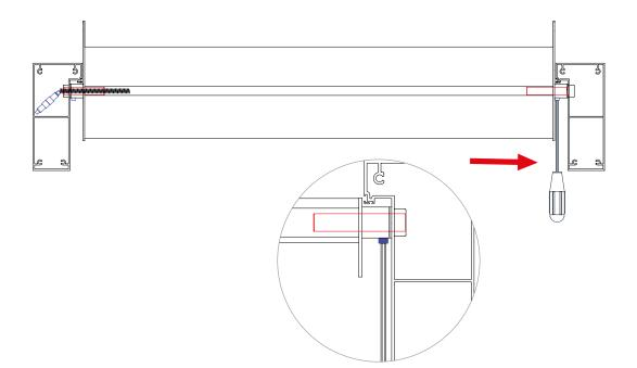
Using a Nº 4 Allen key, pull back the axle until it stops in the grooved hole.
