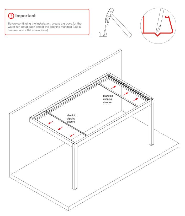
Apply the provided sealant between the contact sides of the **opening** and **closing** beams and their corresponding surface manifolds. Then clip the opening and closing manifolds. You will possibly need to use clamps (jacks) or wooden plugs to help you with the clipping.
