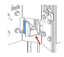
**4.** Press on the 3 sides of the part: bottom, left and right *(marked with red arrows)* to seal the part against the gutter.
