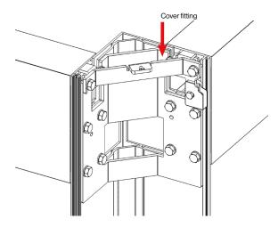
Repeat the procedure with the rest of the beams, placing the column first and then the beam.
