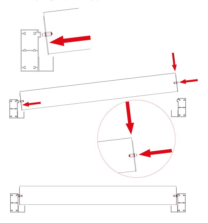
When reaching a hole for LED slats, connect the connector and insert it into the beam (as shown in the images below).
