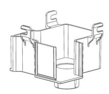
9. Place the collecting tray under the gutter extensions.
