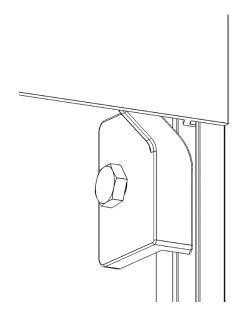
On the left side of the column, clip the profile onto the clipping rubber from the bottom to the top.
