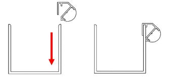
Fit the perimeter LED corner piece shown in the picture on the right to the **corners of the pergola with a column**.
