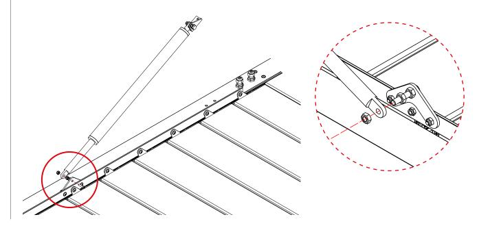
**3.** Move the motor opening the pergola until the bracket can be screwed on the beam threaded holes.
