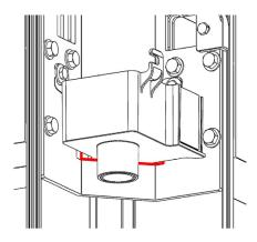
**12.** Finally, fit the drainage pipe to the corresponding collecting trays, according to the descriptions above.
