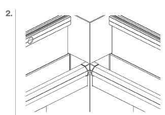
Fit the perimeter LED corner piece shown in the picture on the right to the **corners of the pergola with a mitre**.
