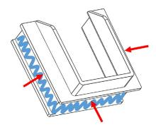
2. Install the piece into the gutter from the inside of the column, taking care not to remove the silicone in the process.
