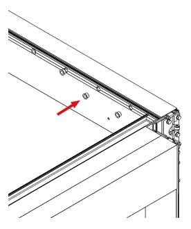
To install the slats without LED you will have a set of O-210 pivot system caps, integrated by a 16,4x25mm plastic cap and a retractable stainless steel axle.
