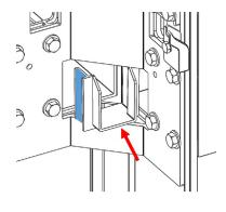
**3.** Once the part has been fitted, it should meet the end of the gutter, as shown in the picture.
