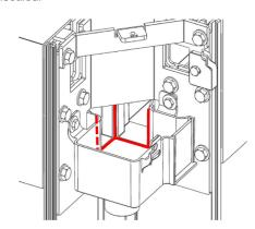
**11.** Seal all possible joints on the parts, aluminium profiles and column reinforcement brackets.
