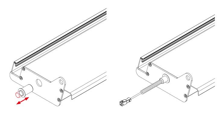
The slats with LED come already pre-installed on one side with a hollow axle. The LED connector comes through this axle and it has a protection spring. The O-210 retractable axle needs to be installed on the other end.
