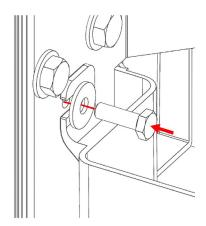
Seal all the joints between the gutter extensions and the collecting tray (marked in red in the picture) with silicone.
