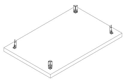
Measure the foundation in order to make sure that the levelling is correct.
