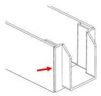
4. Press on the 3 sides of the part: bottom, left and right (marked with red arrows) to seal the part against the gutter.
