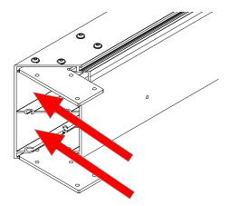
Check that the closing beam is level to the base, its height from the plan and that all markings form a 90° angle with the base brackets.
