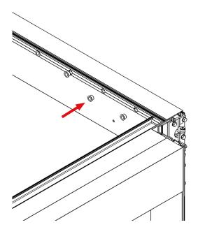
To install the slats without LED you will have a set of O-210 pivot system caps, integrated by a 16,4x25mm plastic cap and a retractable stainless steel axle.
