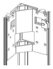
Check that the closing beam is level to the base, its height from the plan and that all markings form a 90° angle with the base brackets. The correct installation of the beam and the bases is critical for the optimum operation of the pergola.
