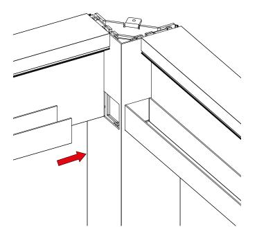
Check that all the "U" profile holes match the M6 machined ones on the beam. If all of them match, apply the sealant between the "U" profile and the beam after screwing the profiles with the USL (ISO 7380) A2x16 screws.
