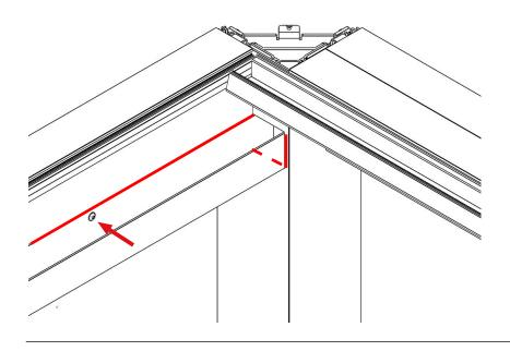
Check that all the "U" profile holes match the M6 mechanised ones on the beams. If they all match, apply sealant between the U-profile and the beam, as well as around the screw holes, then screw the profiles together using ULS (ISO 7380) A2 M6x16 screws.
