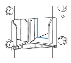
**6.** Repeat the process with the other gutter extension piece if required for the column assembly.
