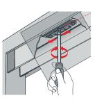
Note: Adjust the thread tension in the middle of the regulator. Please note that too much thread tension can cause the screen to malfunction.
