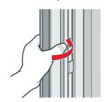
Turn the sliding profile slightly until the hook is released. Hold the sliding profile with your hands in the middle.
