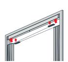
**9.4** Install the second pleated mosquito screen unit above the thread regulator.
