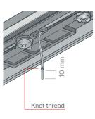
Note: make sure that the thread regulator is not installed in the upper rail screw. If this is the case and you cannot avoid it, cut the thread and make a double knot leaving about 10 mm at the end of the thread as
