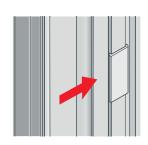
7.2 When the screen is closed, the anchorage is hooked into the sliding bar and the sliding bar is withdrawn firmly towards the folded mesh profile.
