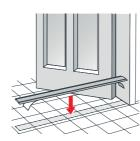
4.2 Remove the white tape from the double-sided tape and press it to the ground strongly in line with the marked line. Be sure to press it toward the side of the folded mesh profile and make sure that there is more than 7.5 mm of space on each side of the side quide.
