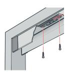
9.3 Install the second pleated mosquito screen unit above the thread regulator.
