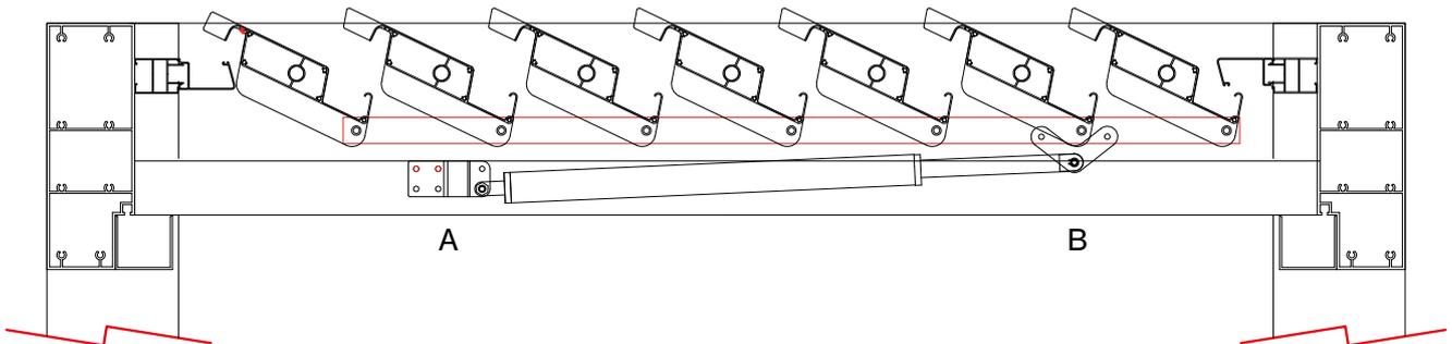
4. Finally we reinstall the motor support in the "U" profile with its 2 screws (A).
