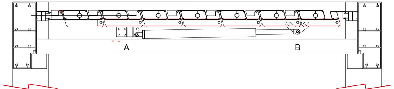
3. Mount the nut on the transmission plate stud so the motor does not come out (B).
