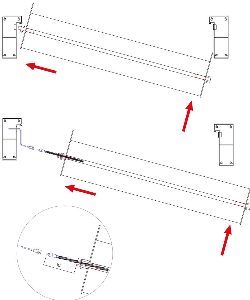
To install the slats, they must be tilted with the end caps facing down, inserting the fixed axle first (left) and then the mobile one (right).
