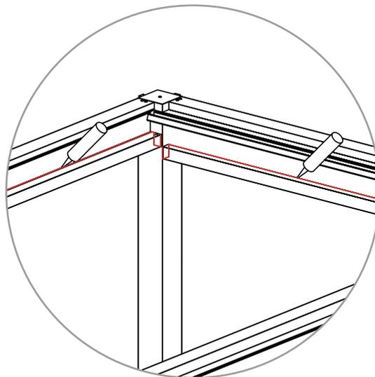
1.10 Drainage channel closed column
