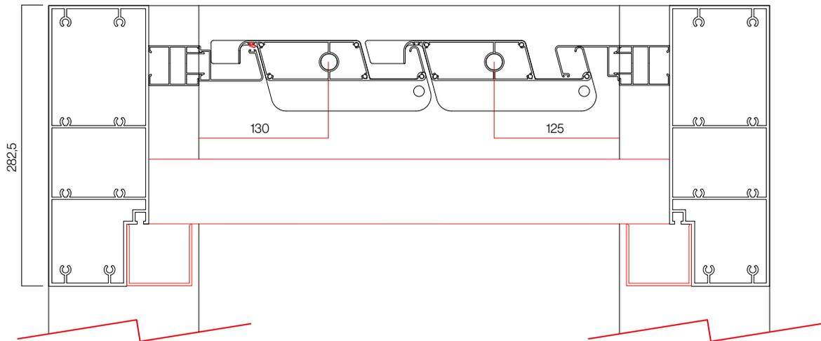
Check that all the "U" profile holes match the M6 machined ones on the beam. If all of them match, apply the sealant between the "U" profile and the beam after screwing the profiles with the USL (ISO 7380) A2x16 screws.
